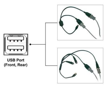
• PRO 0808 / 1616 Using RS-232: Connect RS-232 port to USB port at front/rear of DVR by using a converter.
