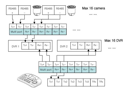
• Please make sure to connect "Tx to Rx "or "Rx to Tx" with positive polarity. (+ to +) and (- to -).
